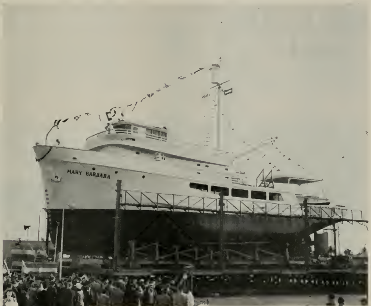
Part of the crowd of over 1000 gathered to see the launching of the Mary Barbara, 106-foot welded steel tuna clipper built by National Iron Works for Serefino Parmigiani and J. E. Mellusi.
